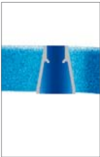
Cast bar construction
