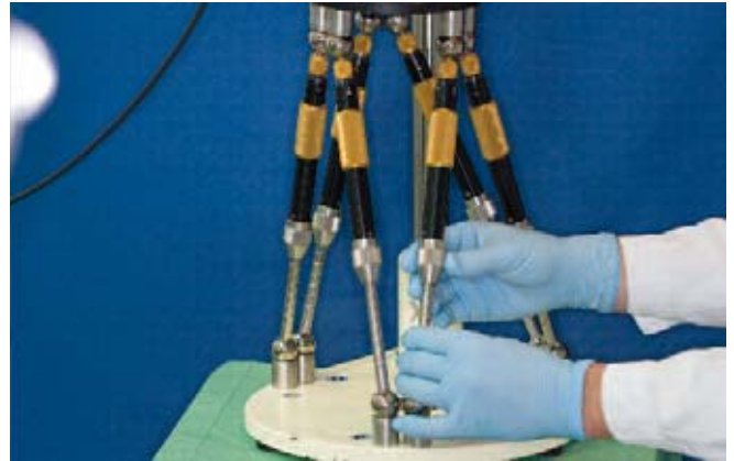
Fig. 37 Adjusting the lengths of the hexapod legs.
