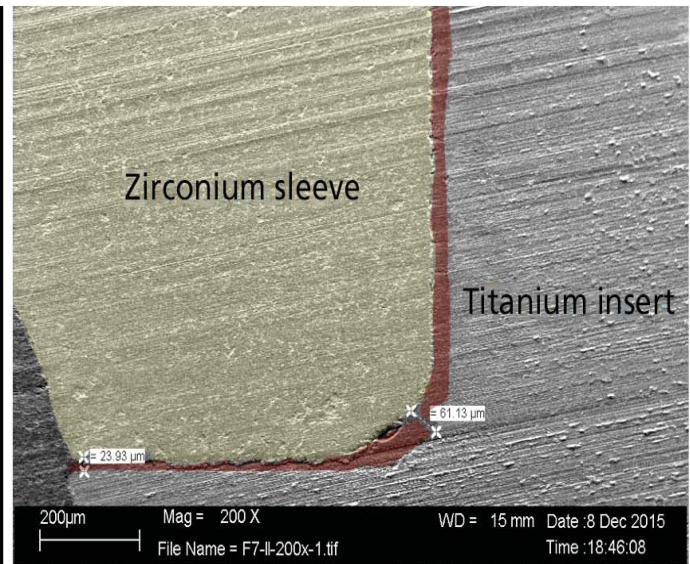
Fig. 2: Magnification of the external bonding gap (L1) with a size of 0.21µm. The gap of the bonding joint is therefore more than half as small as for adhesive mounting of crowns on teeth, where a bonding joint of 50µm is regarded as being ideal.
