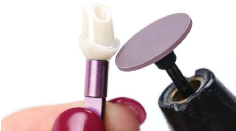
Fig. 6: Reworking of the surface in the basal, submucosal region with special rubber polishers. The desired residual roughness of 0.2-0.4 µm was achieved.
