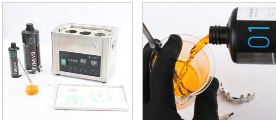
Figs. 10 and 11: Standardized three-stage cleaning process with a washing protocol in the ultrasonic bath.
