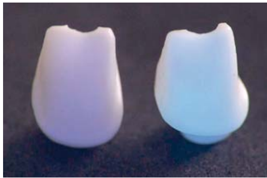
Fig. 31: The sintered abutment left (without) and right with fluorescent solution treatment.
