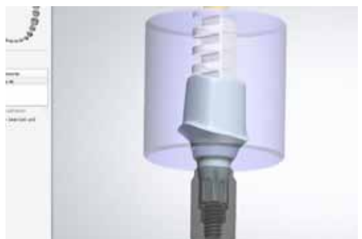
Fig. 22: The milling cylinder is superimposed and the positioning of the abutment checked.
