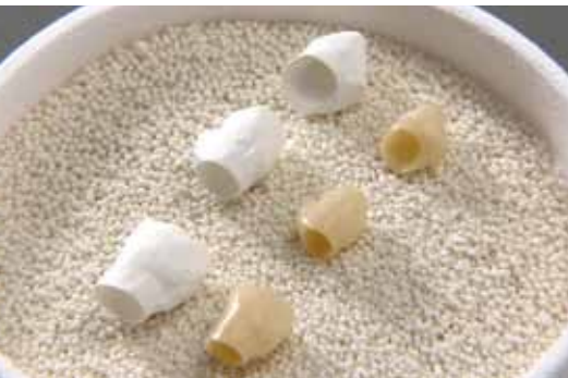
Fig. 36: The unsintered and sintered zirconium oxide caps in comparison: The previously stained ceramic has been shrunk in a controlled manner.
