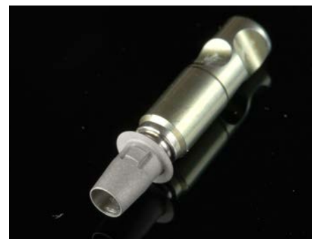
Fig. 25: To bond the hybrid abutment crowns, the iSy Titanium base CAD/CAM were screwed to a lab analog and silanized.
