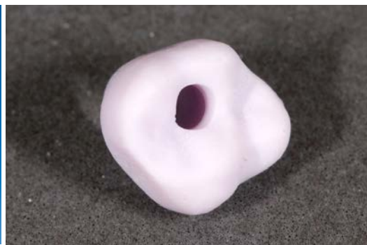
Fig. 26: The anatomic hybrid abutment crown was milled from the lithium disilicate glass ceramic IPS e.max®.
