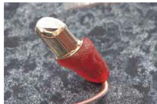
Fig. 28: The screw channel is blocked out, the primary component is coated with conductive silver lacquer to ensure gold separation in the blocked out area.
