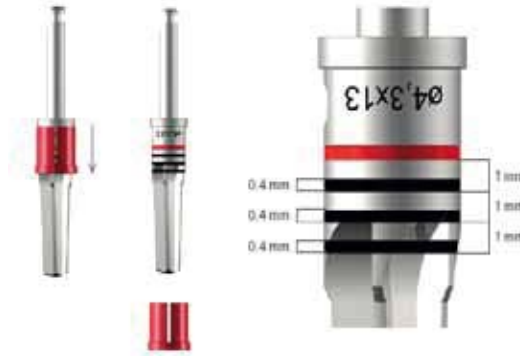
Abb. 8: The shape drill has an optional depth stop which helps to ensure that the implant shoulder is placed 0.4 mm supra-crestally. Additional laser markings are provided for deviating insertion depths, if so desired.
