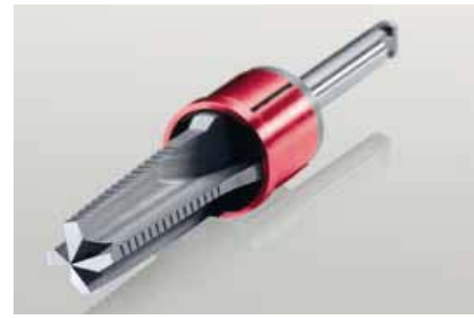
Abb. 8: The shape drill has an optional depth stop which helps to ensure that the implant shoulder is placed 0.4 mm supra-crestally. Additional laser markings are provided for deviating insertion depths, if so desired.
