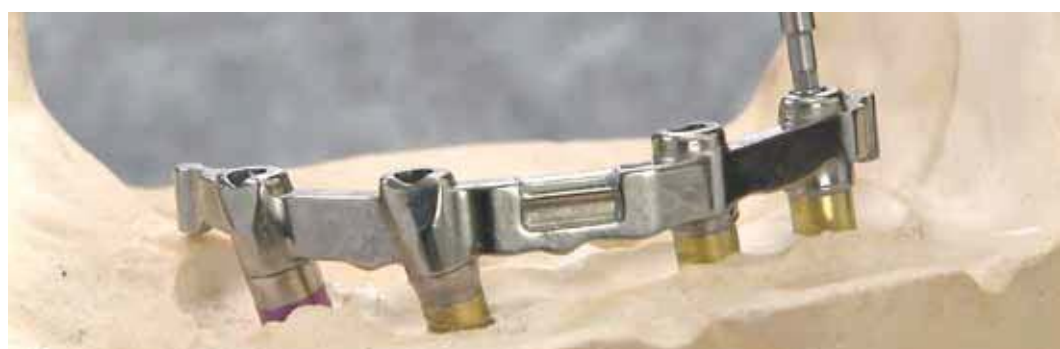
Fig. 35: The fit of the bar, which was also milled externally, is checked on the master model with the Sheffield Test. With one tightened screw in each case, the bar is positioned tension-free on the other abutments.
