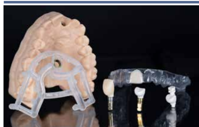
8. The digital design was passed to the DEDICAM manufacturing service. There, the models were manufactured using the 3D printing process, as were the drilling template, gingiva former and impression post, as well as the temporary implant crown. These were delivered after four days and were available for surgical intervention in the dental practice. The deep-drawn splint with acrylic tooth was on hand for temporary restoration in case primary stability proved insufficient.
