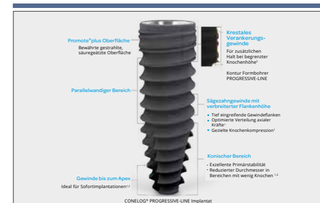
4. The Progressive-Line® Implant with its typical sawtooth thread and deeply engaging thread flanks compresses the soft bone and optimally distributes axially acting forces. Due to the conically tapered apex, insertion is also possible in sites with reduced bone volume.
