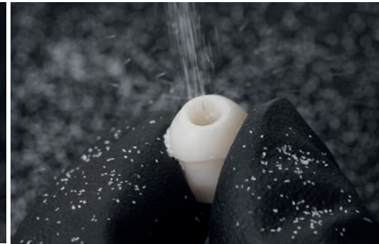
Fig. 7: Conditioning of the inner surface of the zirconium oxide sleeve: blasting with aluminum oxide at 0.5–1 bar // 50 µm.
