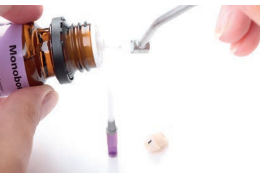
Fig. 8: The bonding surface of the titanium base and the zirconium oxide sleeve are wetted uniformly with Monobond Plus.
