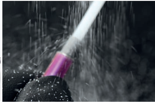
Fig. 6: Conditioning of the titanium base: blasting with aluminum oxide at 1–1.5 bar // 50–110 µm.
