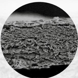
SEM picture of Mem-Lok® Pliable at 50-fold magnification – not side-specific; dense, uniform single layer <sup>[11]</sup>
