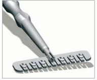
**Pick up the titanium pin** Set the work element of the applicator on the titanium pin head from vertically above, press slightly so that the titanium pin head gets pressed into the work element.
