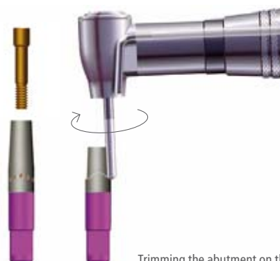
Trimming the abutment on the lab analog
