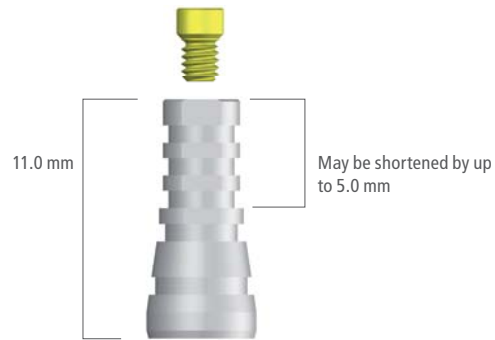
Vario SR titanium cap, bridge, with Vario SR prosthetic screw
